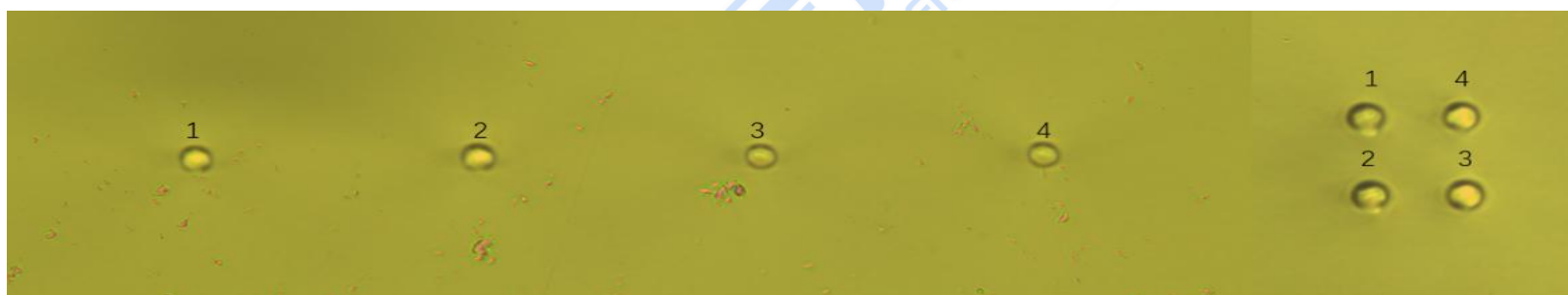
四芯光纤扇入扇出芯片截面 4-core fiber fan-in and fan-out chip cross section:
